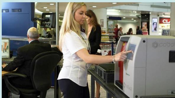
the scanners are widely deployed at EU airports, providing screening of liquids, aerosols and gels (see photo). The handheld portable unit can be deployed to detect hazardous chemicals, explosives and narcotics, for instance by first responders on crime scenes or at environmental disaster zones.
